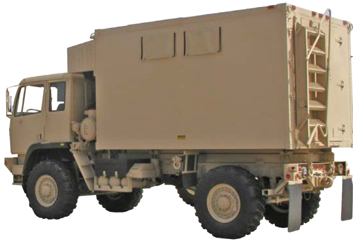
M1079 Shop Van Shelter shown mounted onto a standard 2.5-ton LMTV truck
